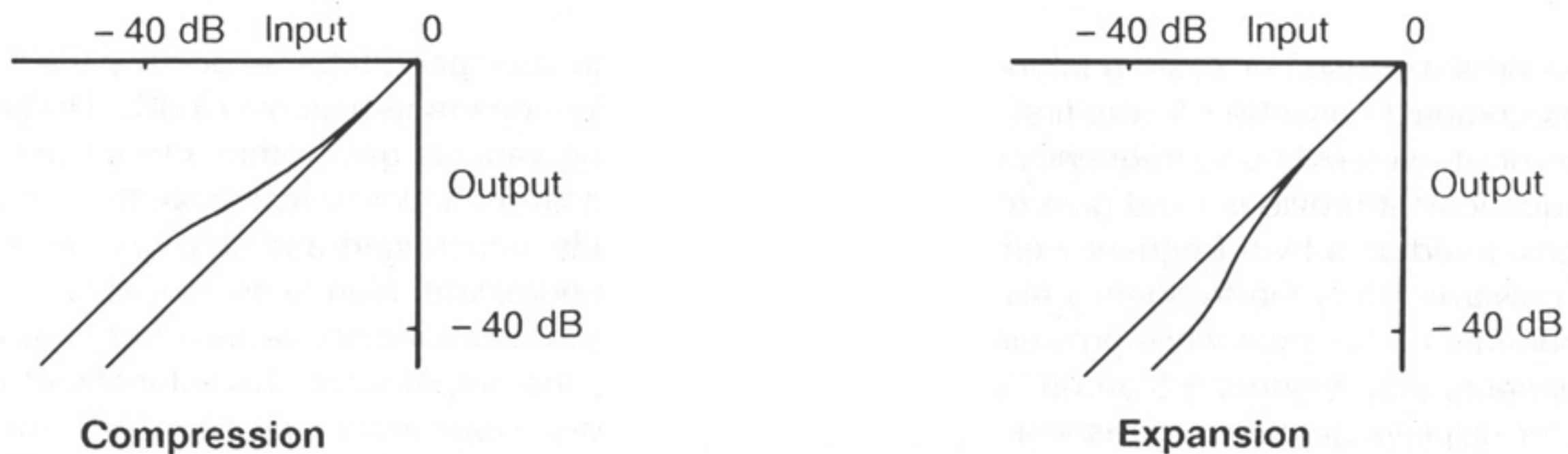
Figure 5.4 General form of compression and expansion characteristic of all Dolby systems
