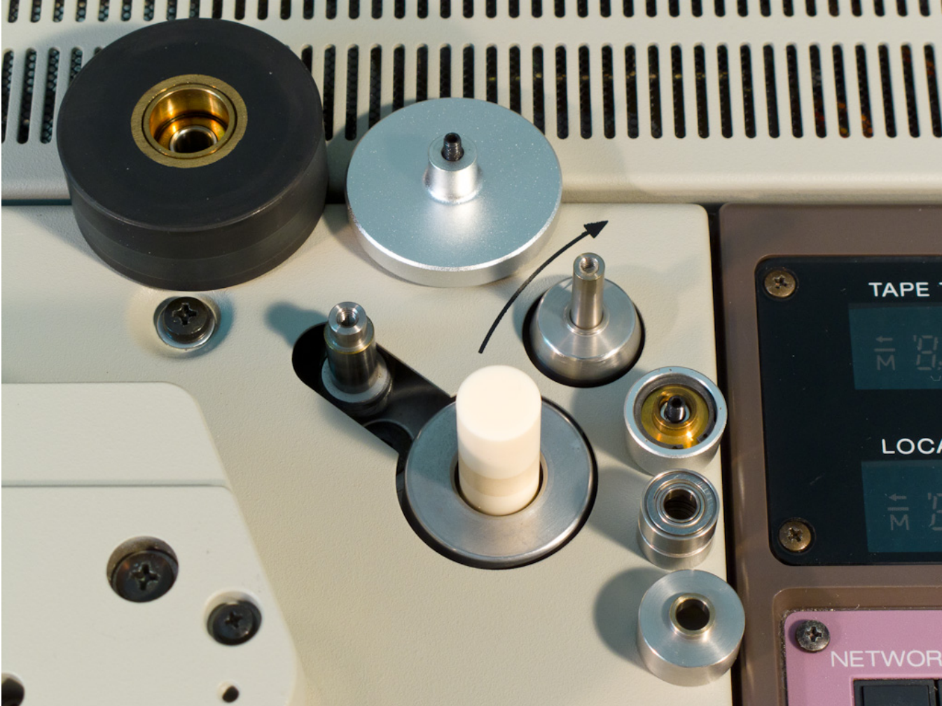
Fig. 14. Pinch roller and T-roller disassembled and removed from shafts. The pinch roller rotates on a 6 mm shaft, the T-roller on a 5 mm shaft.
