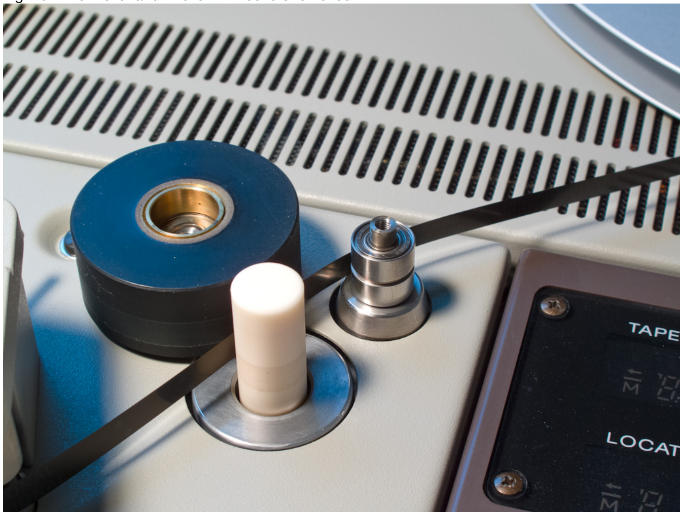
Fig. 13. Pinch roller and T-roller with covers removed.
