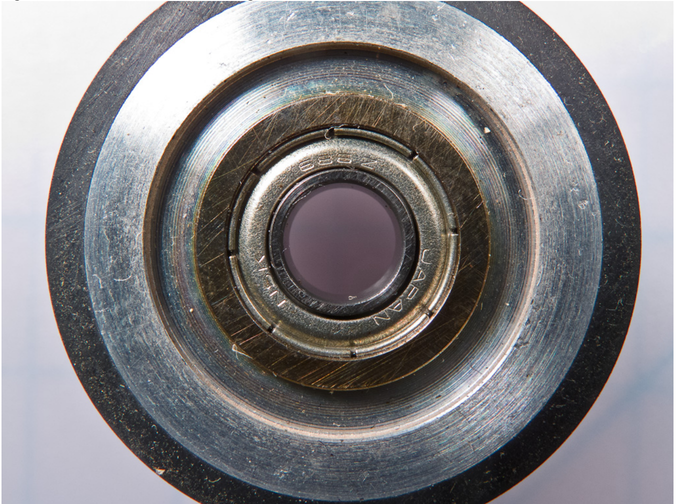
Fig. 11. Timer roller, NSK 686Z bearing detail.
