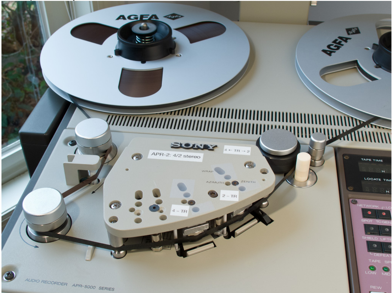
Fig. 3. Tape path as a whole, with the tape moving left to right across the head assembly. Tape speeds are from 4.76 – 76 cm/sec (1.875 – 30 ips), and the largest of the four rollers is only 4.5 cm in diameter, so the rpm are fairly slow. At back left is the first roller, the "S-Roller."
