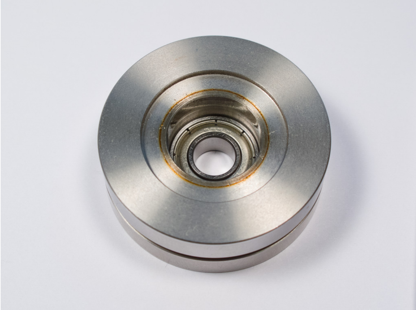
Fig. 5. S-roller interior with upper bearing removed; inner surface of lower 686Z visible. Upper and lower surfaces of the S-roller are identical, with the flange facing out on both.
