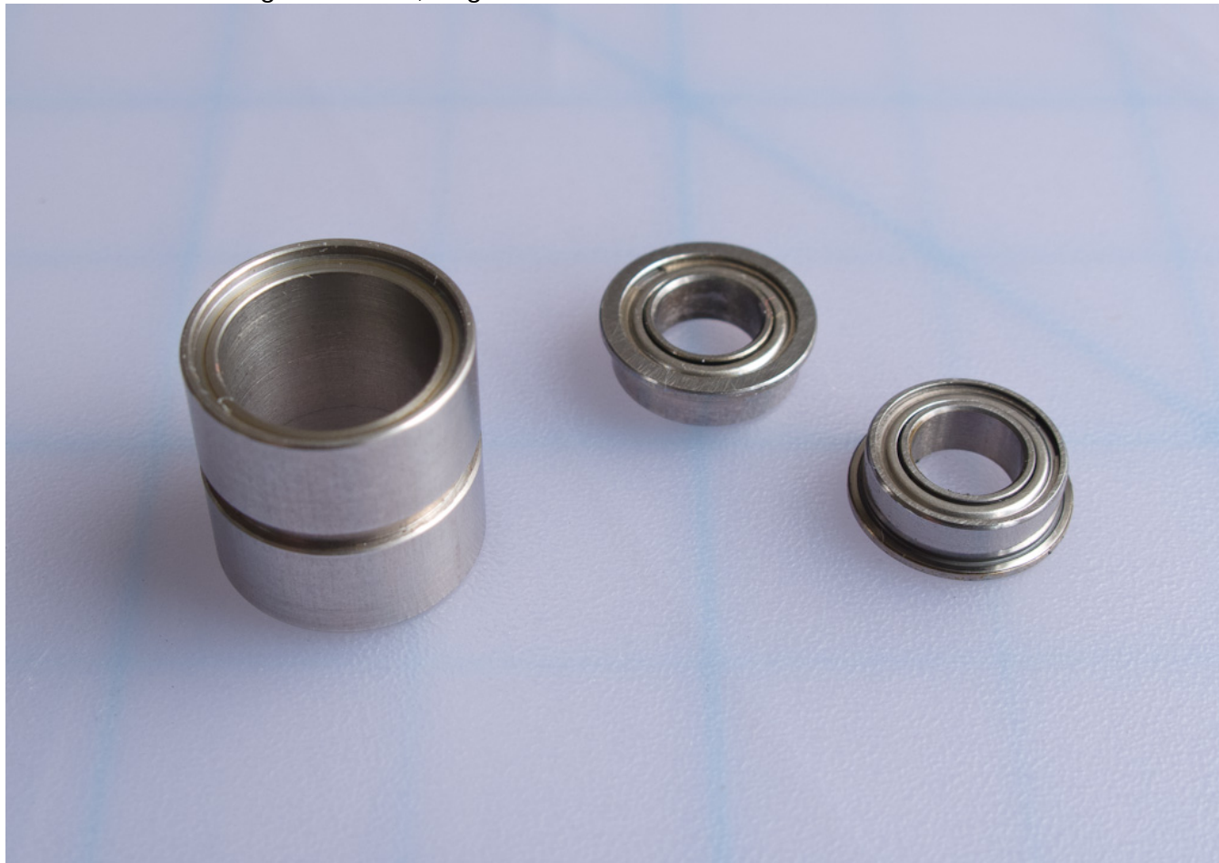
Fig. 17. T-roller bearings removed from T-roller. Bore diameter 5.0 mm, outer ring diameter: 9.0 mm, outer diameter of flange: 10.8 mm, height: 3.0 mm
