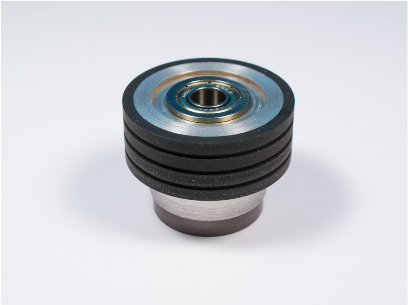
Fig. 9. Timer roller removed from recorder, upper surface.
