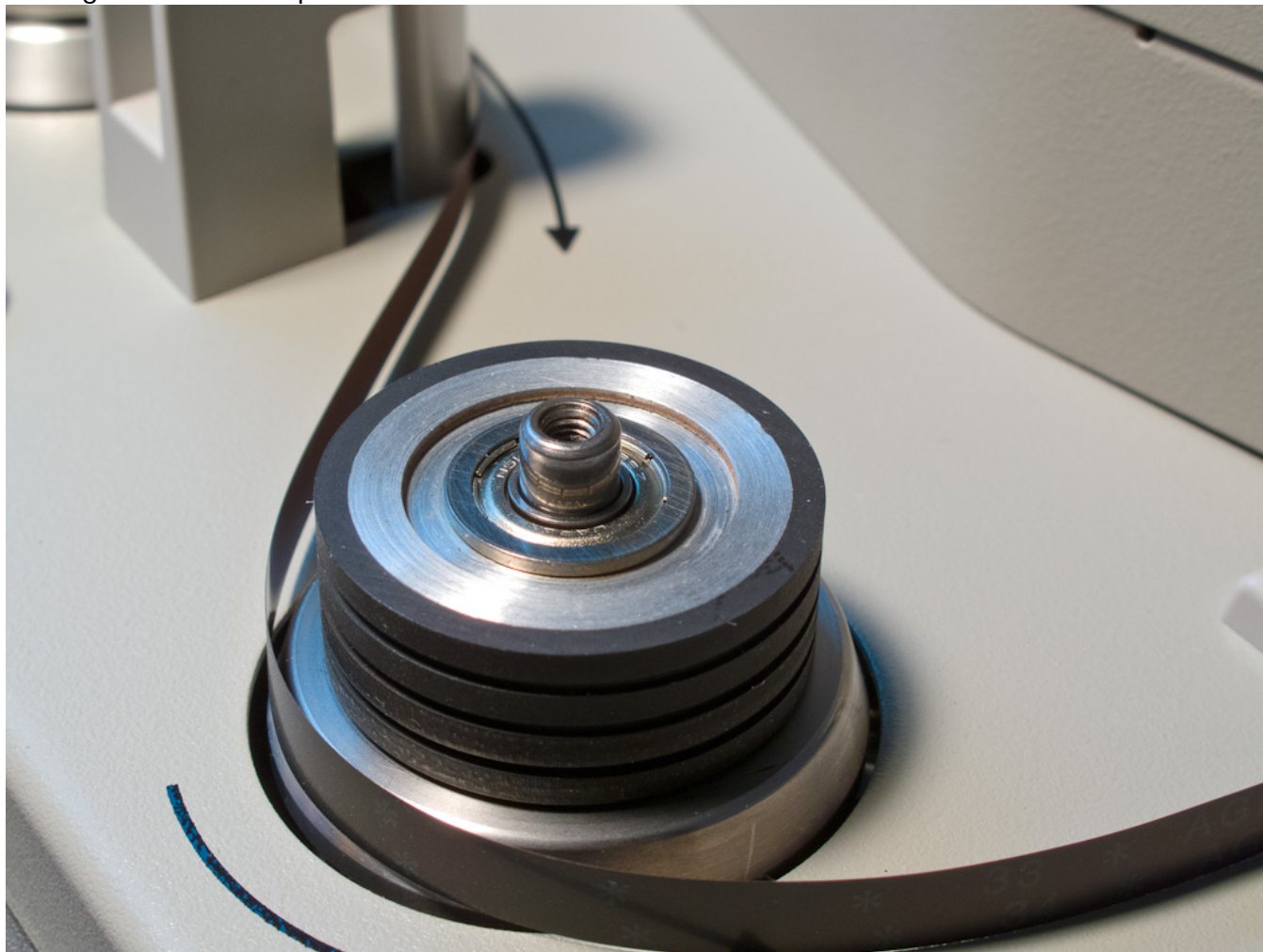
Fig. 8. Timer roller. The Timer roller is a rubber roller covered with a cup and a cap (here removed), which rotates around a 6 mm shaft with two shielded 686Z bearings. Unlike the S-roller, the timer roller bearings are not user replaceable.
