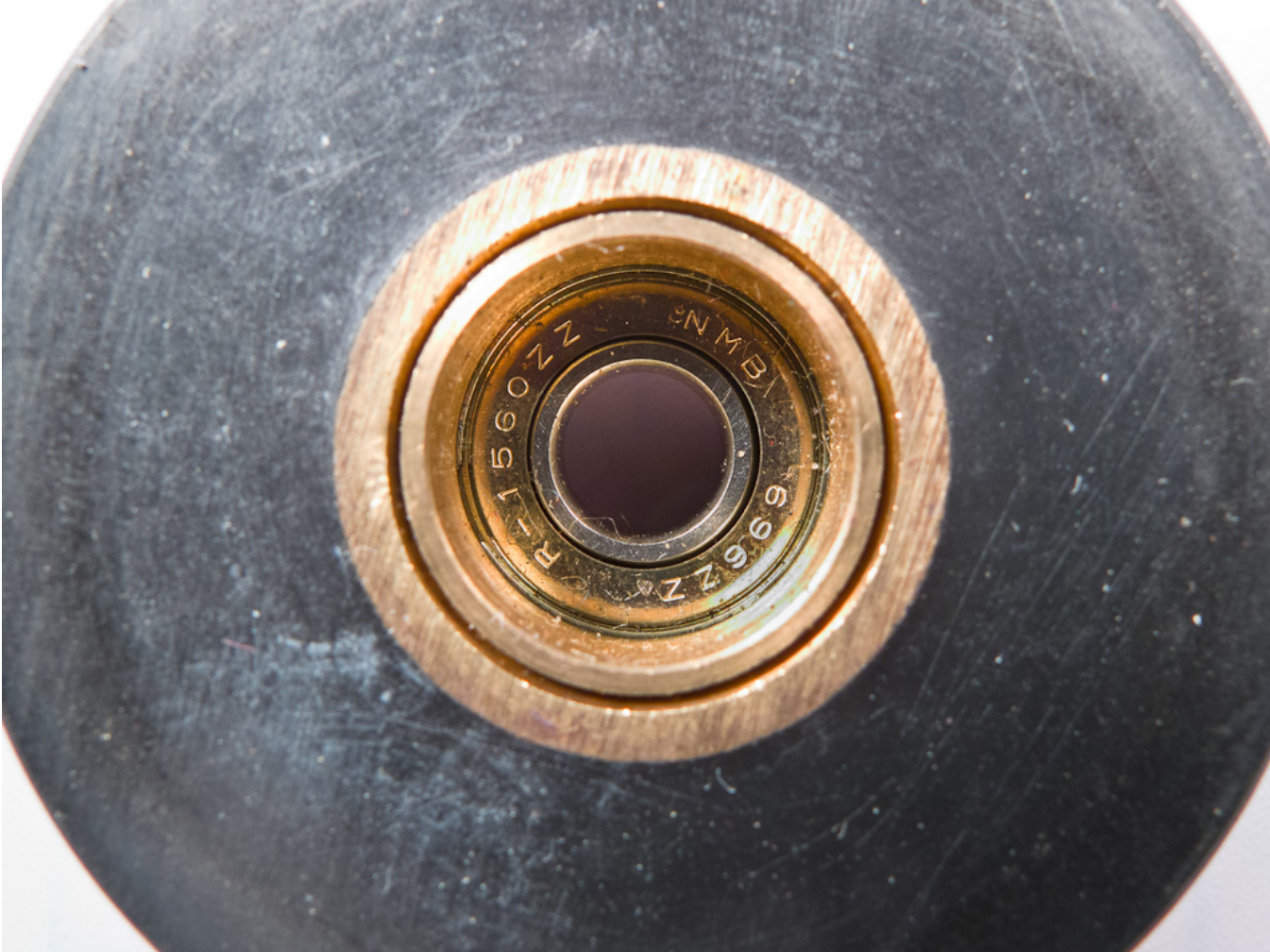
Fig. 15. Pinch roller, upper surface detail: bearing NMB 696ZZ, R-1560ZZ.
