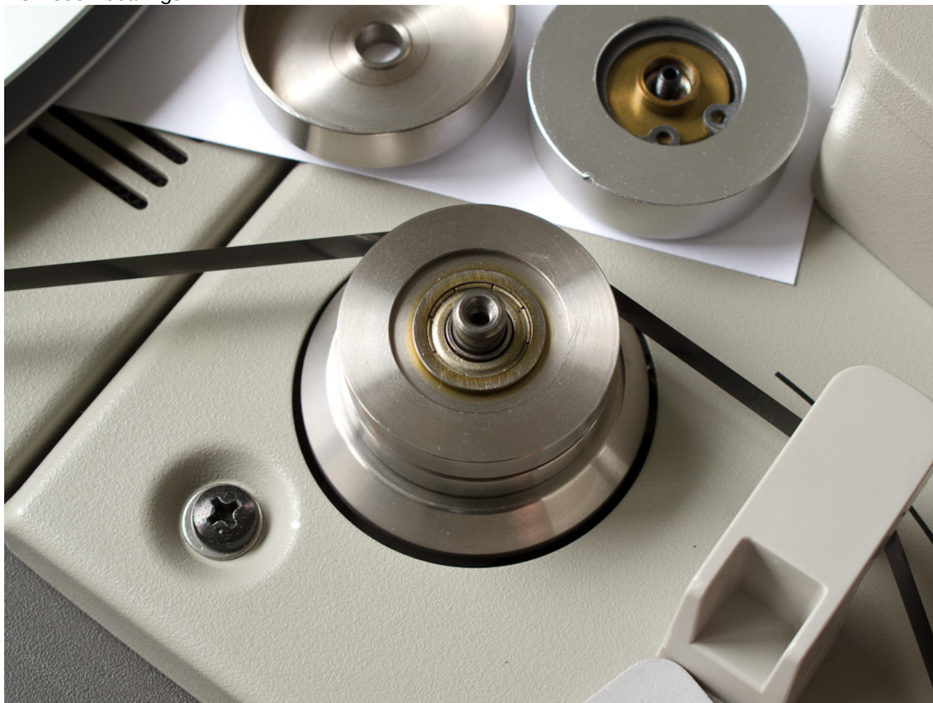
Fig. 4. S-roller. The S-roller is a metal roller and after removing a cup and a cap (shown sitting on a white 4x6 card in the photo below), you can see that it rotates around a 6 mm shaft on two flanged NSK 686Z bearings.
