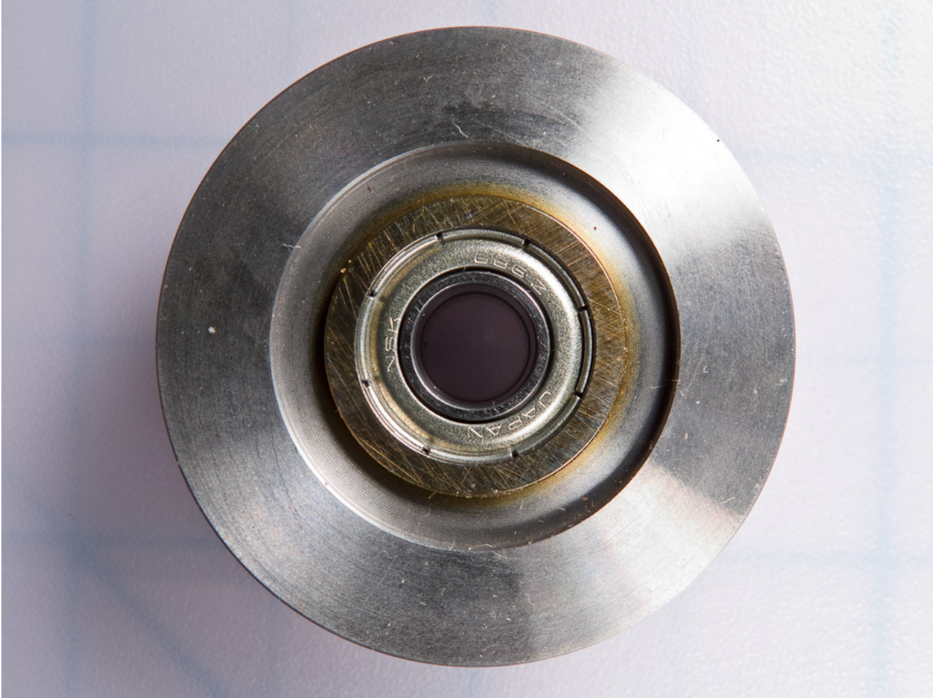
Fig. 7. S-roller, upper 686Z bearing detail.
